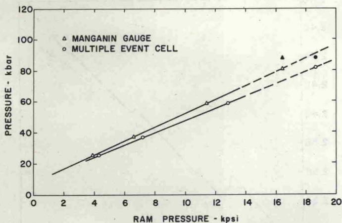
Fig. 5 True pressure versus applied ram pressure calibration curves showing the upper Bi transition at ~81 kbars. The long accepted 88-kbar value is indicated by the dark symbols
