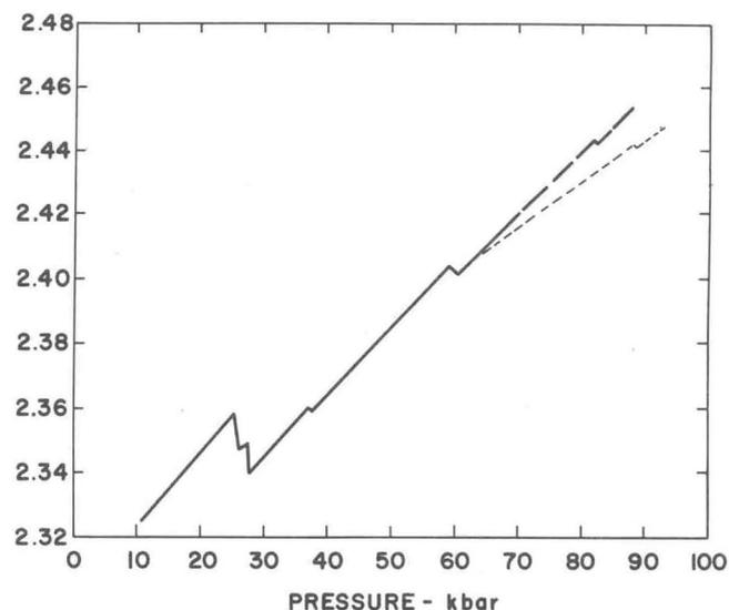
Fig. 4 Resistance versus true pressure curve obtained from the data in Fig. 3 and showing the upper Bi transition at 81-82 kbars
